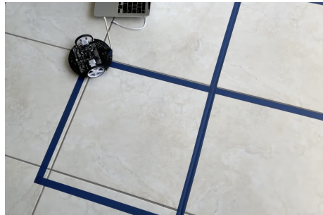
Figure 10: Robot calibration through repeated traversal of square cells
