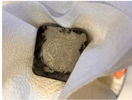
Figure 4: Hydrated mixture in the TPU mold
